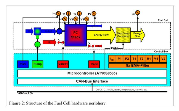
In the test bench (figure 2) all data are measured by the microcontroller (2x temperatures, 2x pressure, 1x current, 1x humidity and up to 10 different module voltages) and will be sent to a PC which sends back the control values to the fan (PWM), pump (PWM), valves (On/Off) and Step Down Converter (PWM). All data will be saved and analysed (Data Logging). First dynamic tests and efficiency diagrams could be realized.
