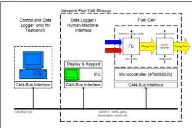
Figure 1: Structure of the Fuel Cell test bench
