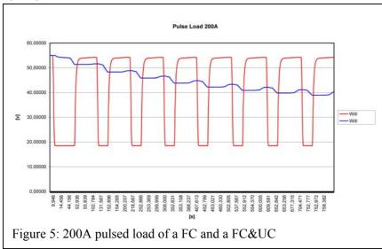
The simulated behaviour of a combined Fuel Cell and Capacitor storage Ultra system (FC&UC) is shown in figure 5, too (blue line). The voltage steps smooth and only a slow voltage reduction cognizable although there is an over load of 11 kW. The dimension of the storage depends on the nominal resp. peak power load and on the voltage range (efficiency range) of the motor.
